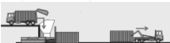
Figure 15 Principles of un-compacted and compacted direct loading in transfer stations 38
