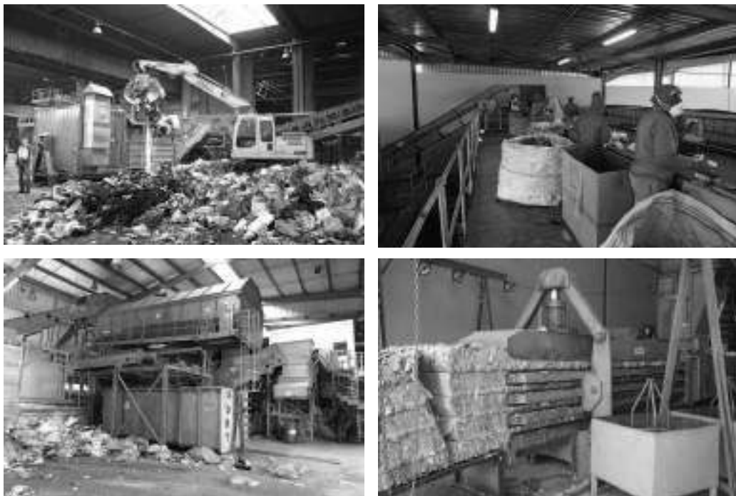
Figure 16 MRF elements: Bunker/bag opener, hand assorting, sieve, baling press 39
