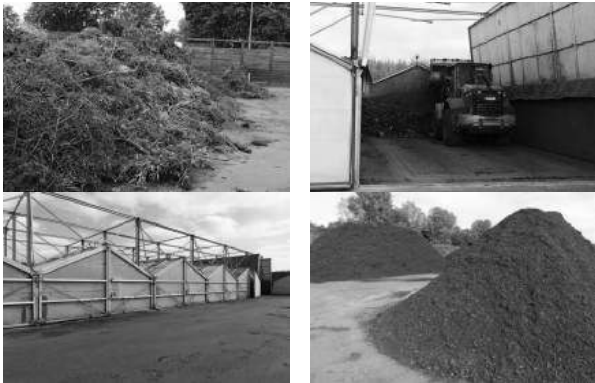
Figure 22 Example composting facility with forced aeration: delivered material, filling of aerated boxes, composting in the boxes, sieved compost 47
